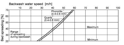
The filter rinsing must be done so that the filter material is in a state of suspension. Only in this way can the held-back substances also be reliably
