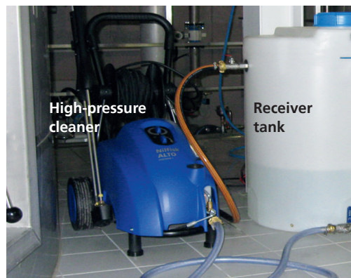
Applying pH-neutral cleaning agents using high-pressure cleaners
