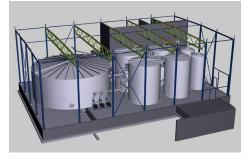
Consisting of two treatment lines with a maximum treatment capacity of up to 550 m<sup>3</sup>/h, the existing system contains an ozone generation system in three lines, three mixing and contact systems, two upright ozone reaction tanks,  $CO_2$  dosing, two alkaline-effect upstream filters for hardening, two downstream filters for bio-filtra-
